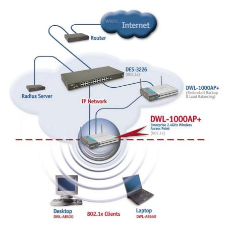
Here is a sample of a network setup using the 802.1x compliant DWL-1000AP+ access point. Your network may look different. For successful communication, you will need 802.1x compliant devices, including 802.1x compliant wireless network adapters. If you are using two or more access points in conjunction for **load-balancing** or **backup**, please remember that IAPP (Inter Access Point Protocol) is passed through the Ethernet connection.
